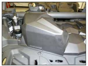
2. Remove the factory intake dust cover by pulling upwards to dislodge it from the mounting grommets.
