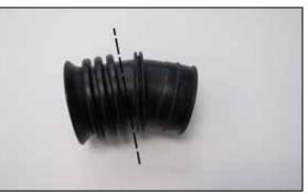
4. If intake kit 57-1141 is not previously installed, remove the factory bellows from the vehicle and trim it where indicated and then reinstall the bellows.
